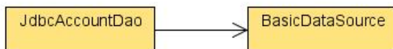
Figure 2 JdbcAccountDao has a dependency on BasicDataSource , which is a concrete DataSource implementation.
