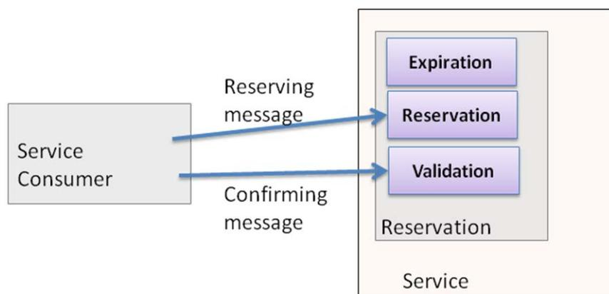
Figure 2 The reservation pattern. A service that implement reservation considers some messages as *reserving*, tries to secure an internal resource, and sends confirmation if it succeeds. When a message considered as *confirming* the service validates, the reservation still holds. In between, the service can choose to expire reservation based on internal criteria.
