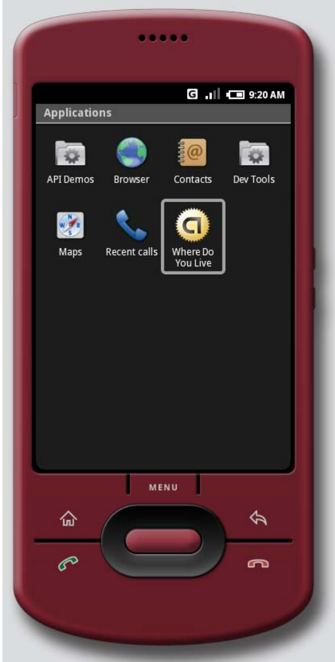
Figure 7 Applications are listed in the launcher based on their Intent Filter. In this example, the application titled "Where Do You Live" is available in the LAUNCHER category.
