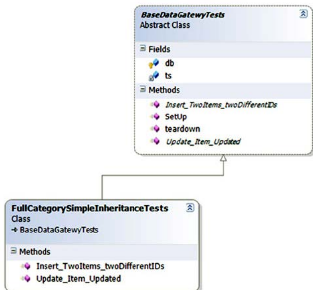
Figure 2 A template test pattern ensures that developers don't forget important tests. The base class contains abstract tests that derived classes must implement.
