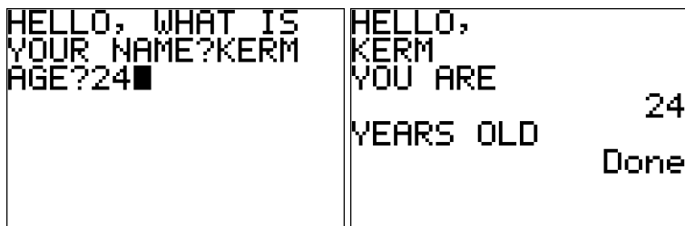
Figure 9 Running the CONVO program. Here, the user enters KERM as the string for his name and number 24 as his age.
