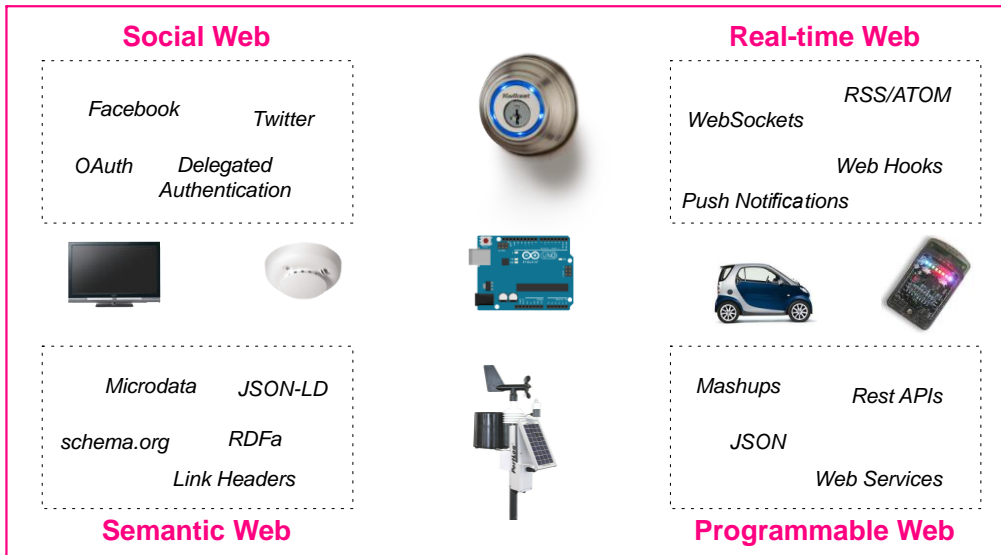
Figure 4 – The Web of Things is the ability to use modern Web standards directly on embedded devices. By leveraging all these standards for IoT scenarios, we both enable new types of interactive applications to be built, and also make sure that devices can be integrated with modern Web applications and services with minimal effort.
